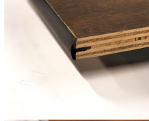
5/8" thick plywood core with Black Vinyl Flush Edging.
